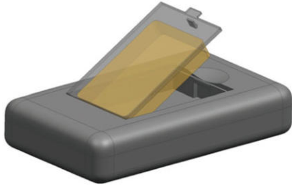
Fig. 10.5 Conceptual illustration of the compartment door of a consumer electronics product
